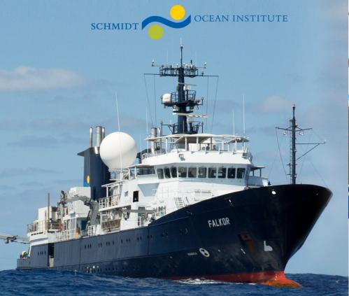
The globally capable 272-foot Research Vessel *Falkor* is Schmidt Ocean Institute's key operational asset; equipped with advanced sonar systems for shallow and deep seafloor mapping, sub-bottom and current profiling, and fisheries studies.
